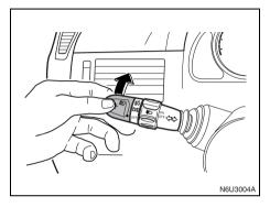
The exterior lamp band has three positions:
